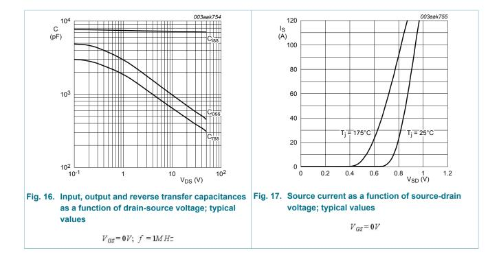
N-channel 100 V 7.6 mΩ standard level MOSFET in D2PAK
